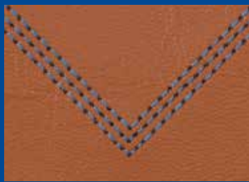
Sewing speed:2,800sti/min, stitch length: 4mm
