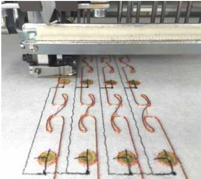
RFID antennas placed and fixed by embroidery.
